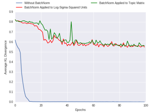
Figure 3: In optimization without any BatchNorm, the average KL gets minimized fairly early in the training. With BatchNorm applied to the encoder unit that produces \log \sigma^2 , the KL minimization is slow and slower if BatchNorm is also applied to each of the topics in the decoder.
